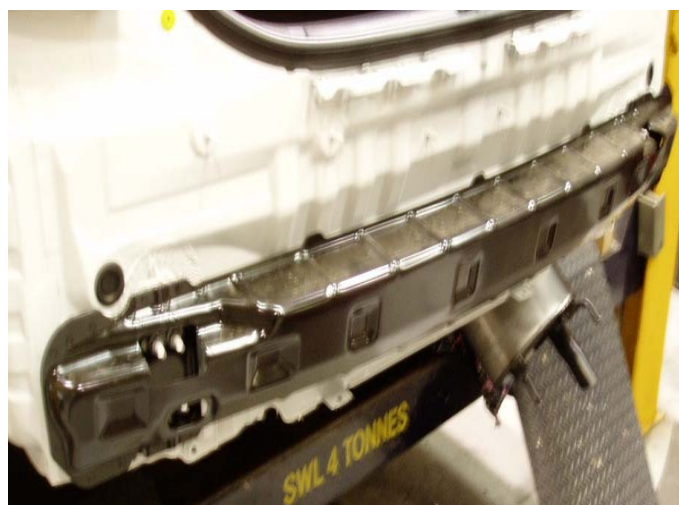
FIG 2: Shows impact beam on car
