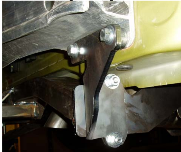
Fig 2: Mounting points of side brackets onto vehicle shown. Figure also shows towbar & bracket being bolted together.
