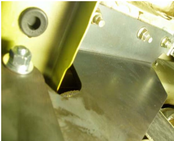
Fig 5: Shows bumper cut-out profile.
