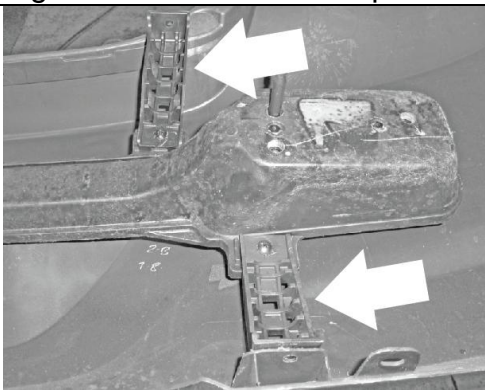
Figure 6 – Remove the impact beam bolts.
