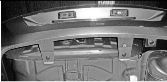
Figure 2 – Remove scrivets from underneath the bumper.
