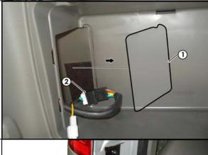
9. From outside the vehicle, remove the two bolts (1) from the LHS rear bumper (2).
