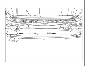
Created a Bumper Cut 70mm wide and 105mm high starting 45mm from bottom edge of Bumper and in centre of the Bumper Bar.
