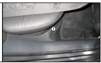
13. On the RHS of the luggage compartment, remove the blanking grommet (1) and drill the hole out to #30mm
