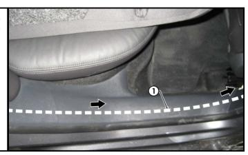
**23.** Continue to route the trailer harness 'ORANGE' power wire along the RHS front scuff plate and up towards the fuse panel.
