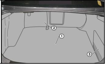
5. Remove the rear trim (1) by first removing the two clips (2).
