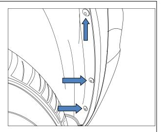
Remove 2 Screws from Bumper Bar which located behind the Wheel Well lining for both the LH &RH side.
