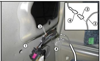
**21.** Route the trailer harness 'ORANGE' power wire (1) along the RHS of the luggage compartment and towards the front of the vehicle.
