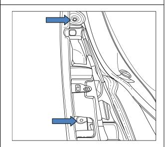
Disconnect Rear Light Plug and remove light by fastening screws located in the Rear Light Cavity in the boot. Then firmly pull on Rear Light to remove.
