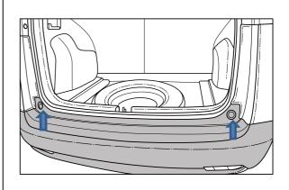
Remove the cover to expose M6 Bolt in the Boot Cavity and then unbolt it from either side.
