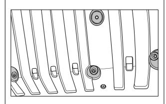
Lower the Exhaust to gain better access as shown by removing the two Muffler Bushings from the Vehicle Pins.
