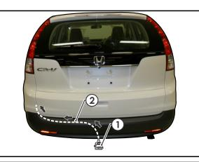
**19.** Connect the tail harness (tail length 1800mm) 8-way connector (1) to the trailer patch mating 8-way connector (2).
