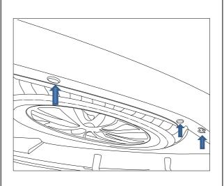
5. Remove 2x Bumper Screws from the Boot Cavity as shown.
