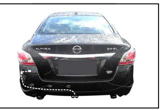
**12.** Inside the vehicle, connect the tail harness (tail length 1200mm) 8-way connector (1) to the trailer harness mating 8-way connector (2).
