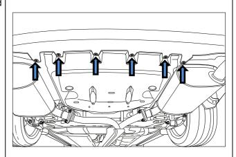
4. If fitted, remove the undercover by removing 5 x flanged Nuts.
