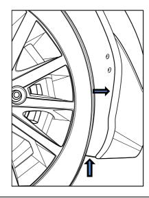
3. Remove 2 x push Rivets and 4 x Screws located on the underside of rear bumper.
