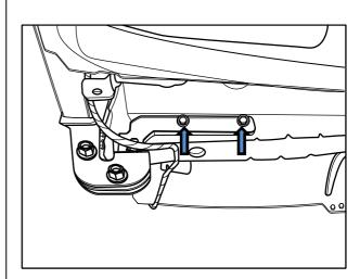
13. Refit any exhaust hangers. Removed in step 8.
