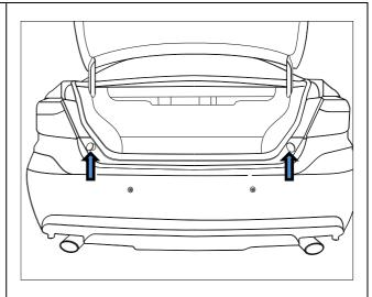
8. Remove and discard 6 x Nuts securing impact beam to rear panel; remove and discard impact beam.
