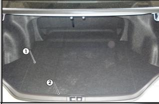
2. Remove the LHS and RHS tool storage compartment (1) and the centre wheel cover (2).
