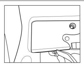
12. Offer the welded Towbar assembly to the vehicle. Loosely secure Towbar assembly mounts to the inner side of the chassis rails using 4 x M8 Bolts (2 per side), complete with 1 x Flat washer per Bolt.
