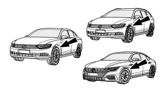
Find the two black connectors in the area shown (Behind the side panel) by pulling them from a foam sleeve and connect them to complete the CAN circuit. Look carefully as they are contained in a foam cover and can be hidden behind another
