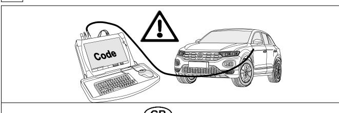
For activation of the trailer function, the coding capability should be clarified / argreed with the respective manufacturer of diagnostic system.
