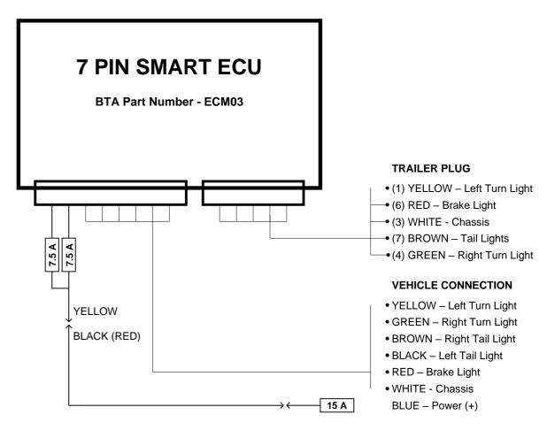
\*\*The blue wire with white connector (Marked 12V) is for the 12 volt power.
