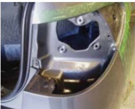
Fig 3; Shows retention points to remove tail lights
