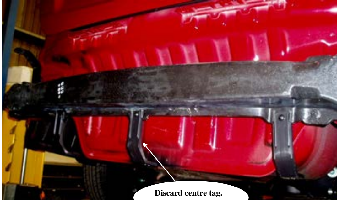
FIG 5: Shows the three bumper tags to be removed.
