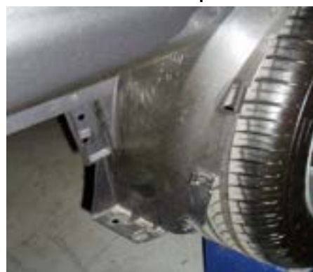
Fig 4: Shows bolts to be removed from under rear arch and underside of bumper on both sides.
