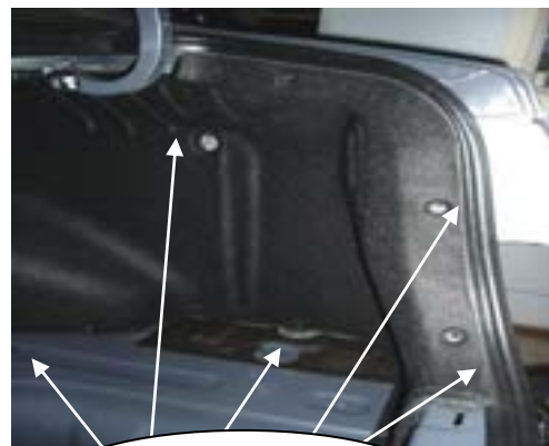
FIG 2: Shows retention points on side panel.
