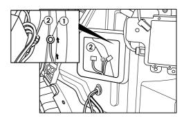
23. Connect the trailer patch connector (1) to the ECU (P/No: 04826) (2). Locate a suitable area on the sheet metal (3) where the ECU will be mounted and clean with an alcohol wipe (not supplied). Remove the backing from the back of the ECU and mount the ECU (2) onto the sheet metal area (3). Ensure the ECU is mounted with the connector pointing downwards.
