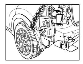
22. Inside the LHS rear quarter vent cavity, secure the trailer patch ground ring terminal (1) to the vehicle grounding point (2).
