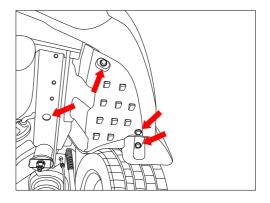
8. Remove 2 x bolts securing the impact beam to the rear panel, accessible from under the vehicle.
