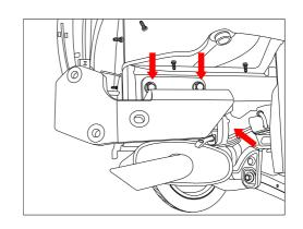
11. Lift cross tube to the side arms and loosely secure each side with 3 x M12 bolts complete with 2 x washers and 1 x nut per bolt.
