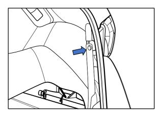
7. From underneath loosened carpet remove 3 x nuts from rear of taillight and remove light assembly.
