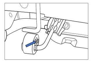
15. Loosely bolt side arms to chassis rail using 2 x M12 bolts & washers on both sides.
