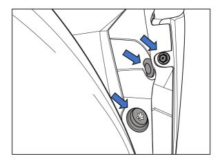
2. On the underside of bumper to back panel remove 2 x push rivets securing the bumper to the back Panel.
