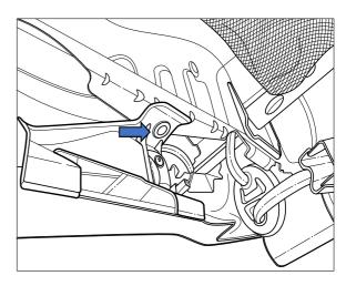
3. Open boot, remove inner carpet and polystyrene Inserts. Remove 4 x push rivets 2 each side attaching inner plastic trim to rearwards face of inside boot cavity.
