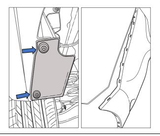
11. Disconnect both exhaust hanger rubbers from rear impact beam.
