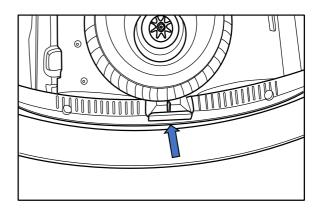
6. Remove 2 x small plastic push rivets in newly exposed area securing inside carpet to chassis rail.
