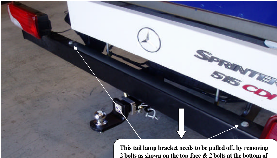
Fig 1: Vehicle with towbar fitted shown.
