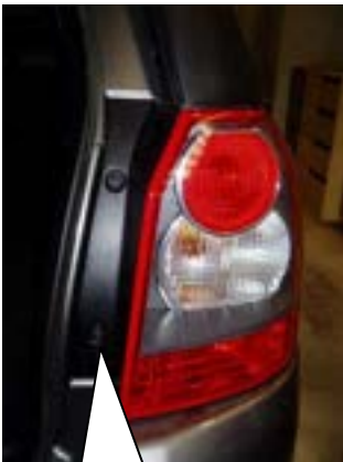
Figs 1 remove taillight assembly.
