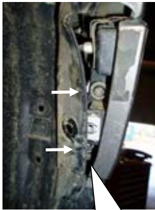
Figs 2 remove torx screws
