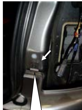
Figs 3 remove torx screws
