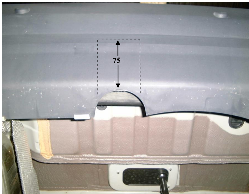
Bumper cut diagram 2. 75mm to be measured around the outside of the bumper
