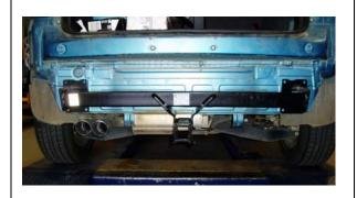
10. Offer towbar to chassis rails and loosely secure with 6 screws from rear impact beam.
