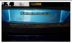
3. Remove 2 torx screws be hide number plate display.
