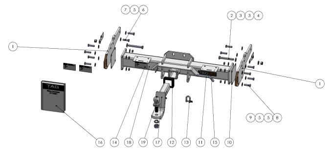
Tools required: 18mm Spanners and or Sockets, 33mm Socket, Torque wrench, Impact Wrench
