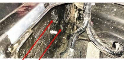
Disengage the clips to separate the step cover from the bumper body.
