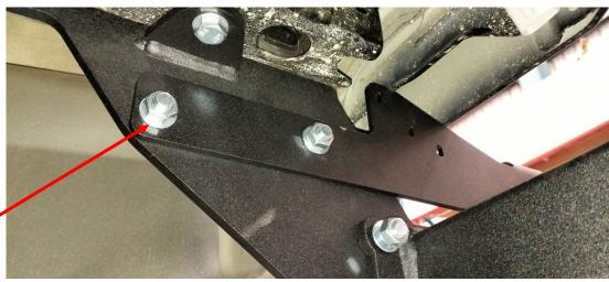
Loosely fasten the bumper bar with new mounts to the inside of the towbar endplates with 2 x M12 x 1.25 x 30 bolts, flat washers and nuts per side.
